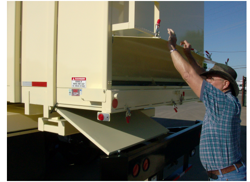
CLEAN OUT DOORS
